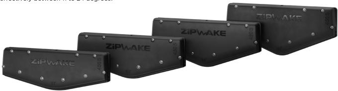
V-shaped centerline mounted interceptors can be included in new installations, or retro-fitted to already installed systems. The modular design enables boat designers to develop their own novel applications, e.g. in multihulls or stepped highspeed craft.
